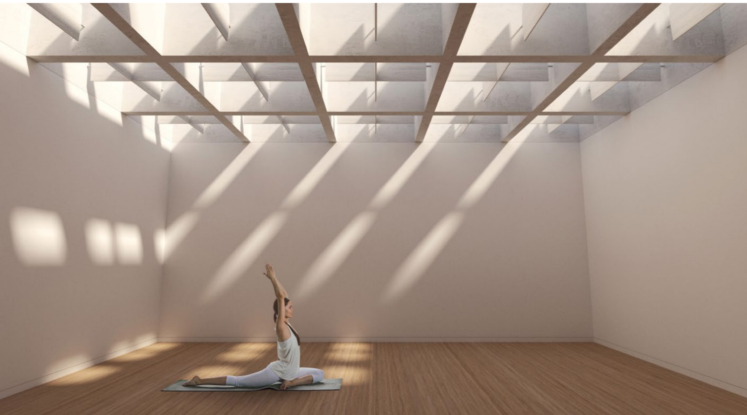
The main Yoga studio, also suitable for Tai Chi, Capoeira and similar physical activities. A major grid of concrete and a minor grid of white-stained timber fins softens the light and adds privacy.
